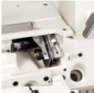
\*Since the looper thread cam is mounted on the shaft, which is separate from the hook driving shaft, the cam is easy to detach.
