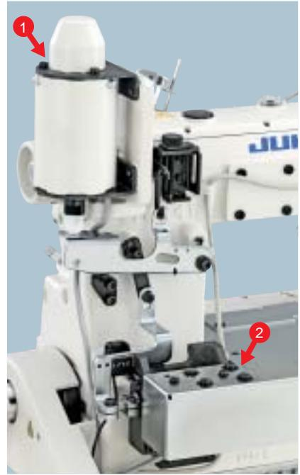
① Presser lifter drive mechanism
