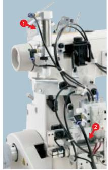
Presser lifter drive mechanism
