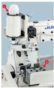
Presser lifter drive mechanism
