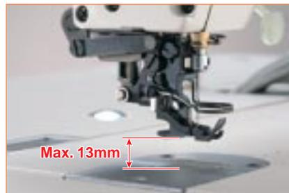
The thread trimmer cuts threads with high to low thread counts without fail.
