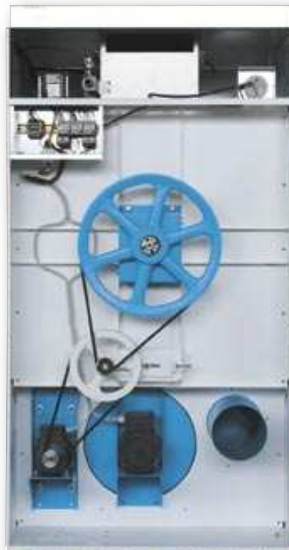
Reversing drum is standard on models ES 23-34-55
